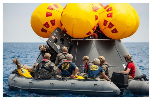
NASA, Navy, and Air Force personnel practice Artemis recovery procedures in the Pacific Ocean as part of Underway Recovery Test-10 off the coast of San Diego. In this photo Navy divers are seen entering the Orion Crew Module Test Article to prepare to practice recovering astronauts out of the spacecraft and onto an inflatable "front porch" where the crew will be picked up with helicopters and lifted up via helicopter back to the recovery vessel.
